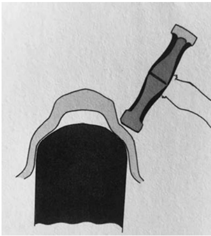
Fig 7 Back raising, from Frances Loyen, The Thames and Hudson Manual of Silversmithing , London, 1980.
